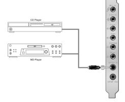
Plug the optical TOSLINK adaptor into the S/PDIF-In combo connector. Then, connect your MD/CD/DVD player's S/PDIF out port to the optical adaptor with the TOSLINK optical cable
